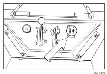
Depress the control for disengaging the mower deck
